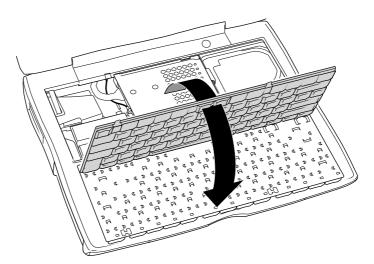
7 Touch a metal surface inside the computer to discharge any static electricity.
