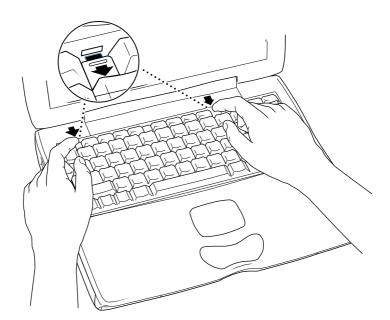
5 Lift the top portion of the PowerBook keyboard up slightly near the top row of keys and pull it back far enough to release the small tabs that hold the bottom of the keyboard in place.
