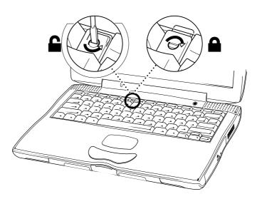
4 Release the keyboard by pulling down on the keyboard release tabs (located to the left of the F1 and F9 keys) until the top portion of the keyboard pops up.
