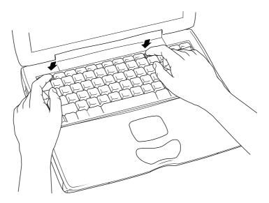
4 Let go of the keyboard release tabs to secure the keyboard in place.
