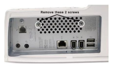
Unscrew these two screws from the rear port panel on your system. This will release the fan from behind the heatsink and allow you to unhook the rear heatsink clips in the next step.
