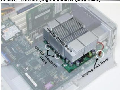
Remove the heatsink from your logic board. Use the needle nose pliers to unhook the clips from the processor card. If your system includes a processor fan or cover, unplug it and then remove by unclipping it and pulling straight up and out.
