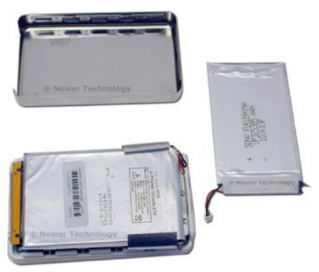
Insert the replacement high-capacity battery onto the logic board socket, it will only plug in one direction. Then, place the battery back onto the adhesive strips, centering it's position on the iPod as shown. Tuck the wires in neatly to the top of the battery, making sure they do not protrude from the inside of the case.
