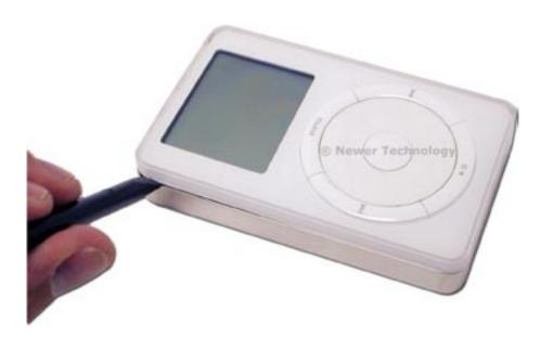
Using the included nylon screwdriver tool, gently insert the pointed end between the metal back casing and the acrylic front of the iPod, at the top of the unit as shown.
