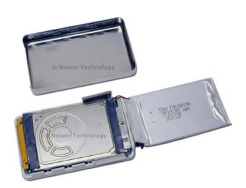
Gently work the battery from the iPod, there are 2 black adhesive strips on the top and bottom of the battery to release. If they stick to the battery, simply peel them off and reapply them to the top of the hard drive as shown here. It may take some force, and you may use the nylon tool to pry the battery off, using gentle force.
