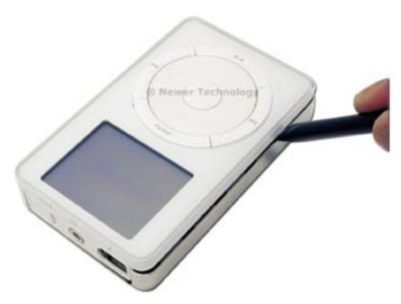
Using a gentle prying motion, work the nylon tool down the length of the iPod toward the bottom as shown. The concealed clips will release as you slide the tool down the iPod's back shell.
