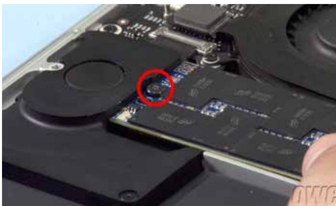
**12.** Reconnect the battery by gently pushing the connector back into its socket and then covering it with the tab.
