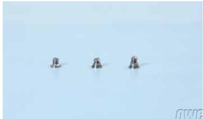
2. To access the inside of the MacBook Pro there are 10 Pentalobe screws to remove from the bottom cover. There are 3 different lengths for these screws so be sure to separate them as they are removed so that they are easier to replace later on.
