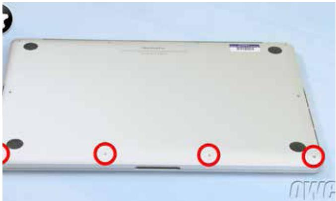
6. The bottom cover can now be removed. Starting near the hinge edge, simply lift up on the bottom cover and set it aside.
