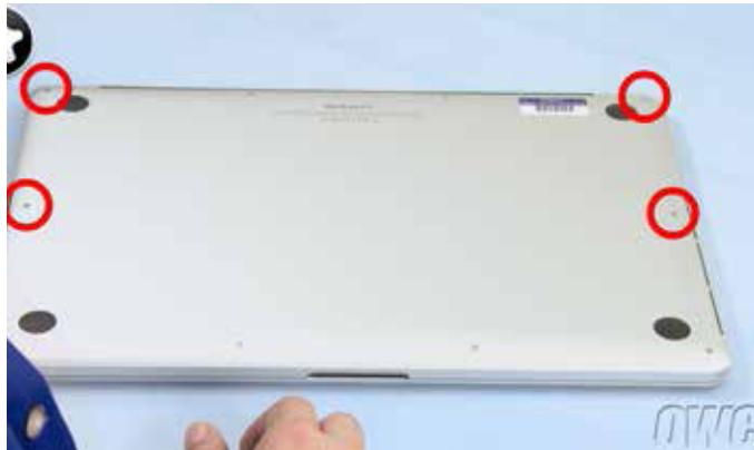
5. Finally, remove the 4 bottom screws. These screws are medium sized compared with the other screws.
