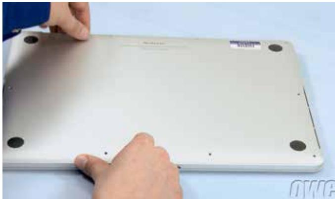
The Solid State Drive is located near the side of the system.
