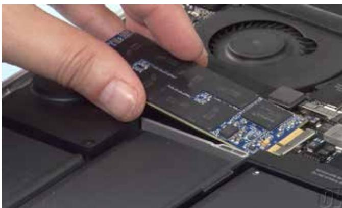
**11.** Secure the drive in the bay using the Torx T5 screw that was removed earlier.
