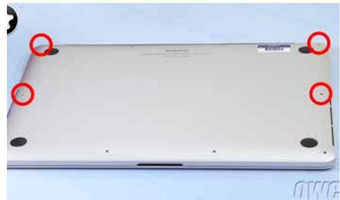
**16.** Finally, replace the 4 medium Pentalobe screws along the bottom.
