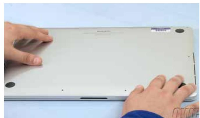
**14.** Next, secure the bottom cover starting with the 2 shortest Pentalobe screws.
