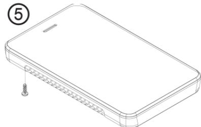
Remove the 2 Phillips screws from the included plastic bag and insert them through the bottom of the enclosure.
