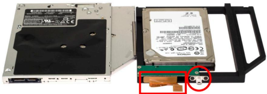
Place the optical drive you removed from your laptop and the hard drive that you already installed into the OWC Data Doubler bracket on the table in front of you as shown.
