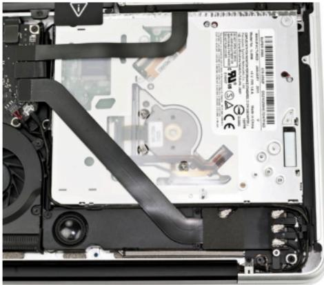
After you've taken the bottom cover off of the computer, you will see the optical drive that you will need to remove to install the OWC Data Doubler.
