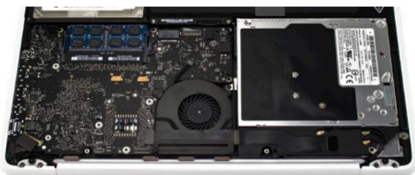
Once you have the final screws removed, you can lift up on the optical drive from the area near the ribbon cable and gently wiggle it out of the chassis.
