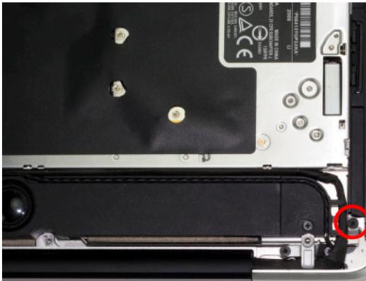
Beginning on the right side of the optical drive (the side closest to the outside edge of the laptop), remove the 2 Phillips screws circled in red.
