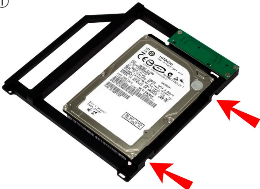
Attach your hard drive to the green interposer board via the SATA drive connection, and then use the two large screws included in the kit to attach the drive to the bracket. Make sure the screws are firmly tightened.
