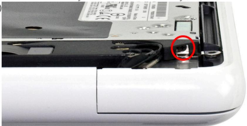
On the right side of the optical drive there is a small black Phillips screw that goes through a covered, black plastic housing and into the optical drive. Remove this Phillips screw. You will be replacing this short Phillips screw with a longer one in a future step.
