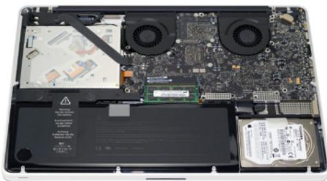
After you've taken the bottom cover off of the computer, you will see the optical drive that we will need to remove to install the OWC Data Doubler.
