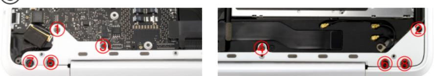
Reinsert the 4 Phillips screws that you removed from the rear vent in the order above - tightening only enough to get the screws started until all 4 are inserted. Then, tighten firmly.
