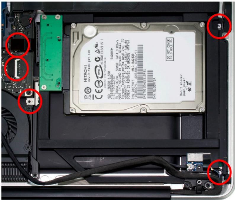
Installation of the OWC Data Doubler bracket with it's hard drive is the opposite of the disassembly process.
