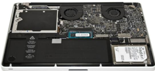
After you've taken the bottom cover off of the computer, you will see the optical drive that we will need to remove to install the OWC Data Doubler.
