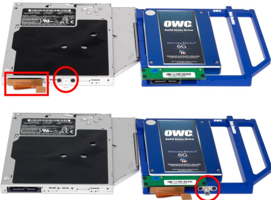
Place the optical drive you removed from your laptop and the hard drive that you already installed into the OWC Data Doubler bracket on the table in front of you as shown.
