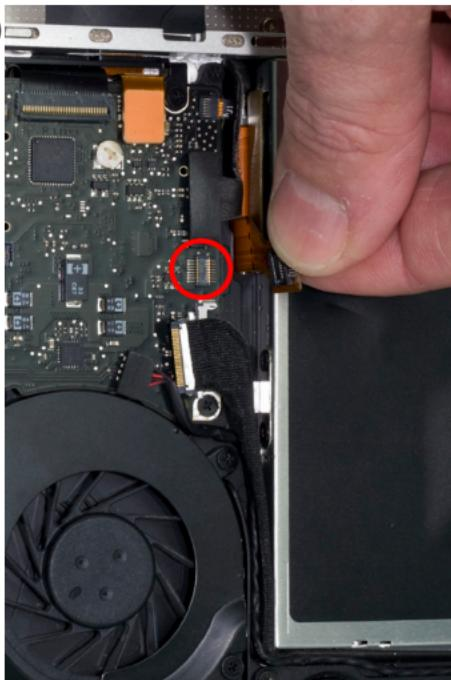
Above the cable you removed in step 7 you will see an orange or black ribbon cable that connects to the optical drive. You need to lift up gently on the cable using a fingernail to release it from the connector on the logic board.
