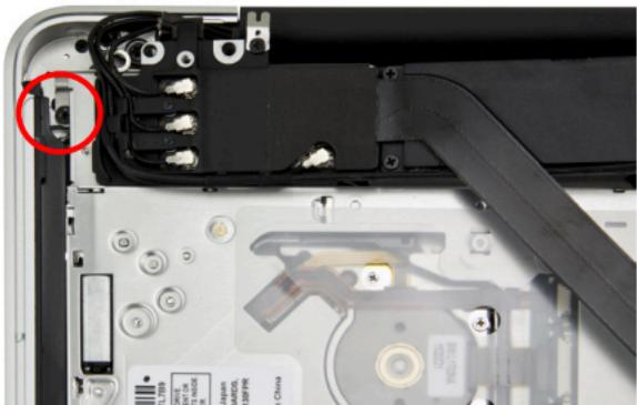
Gently lift the Airport cable assembly up and away from the corner of the computer to expose a Phillips screw that secures the optical drive into the chassis. Remove it.
