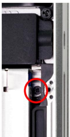
**④** Using a Torx T8 screwdriver, remove the bracket that is above the Phillips screw you want to remove. Once you have the bracket off remove the Phillips screw.
