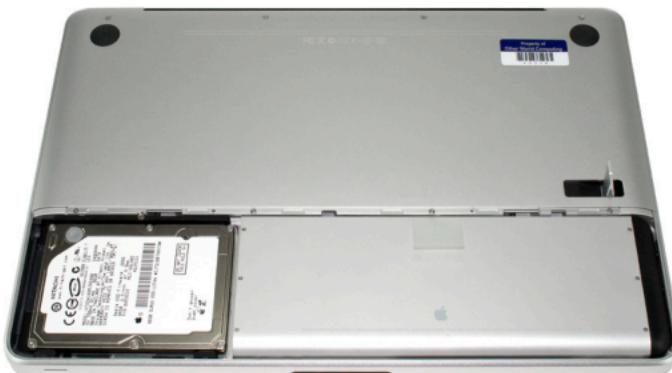
Remove the battery cover from your laptop by lifting the release lever and taking the metal cover off.
