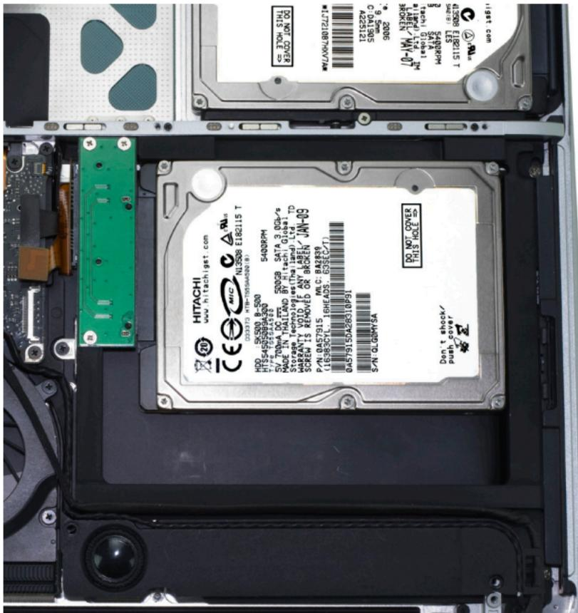
Here you see the OWC Data Doubler bracket inserted into the optical drive bay. 3 screws are inserted but the ribbon cable is not attached to the logic board yet, and the black cable is not plugged in either. Make certain all wires are routed where they originally were before replacing the bottom cover.
