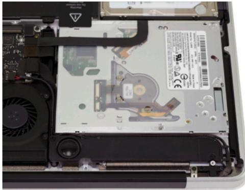
After you've taken the bottom cover off of the computer, you will see the optical drive that you will need to remove to install the OWC Data Doubler.
