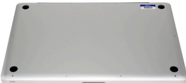
Remove the 10 screws that secure the bottom cover onto the laptop using a Phillips P0 screwdriver.
