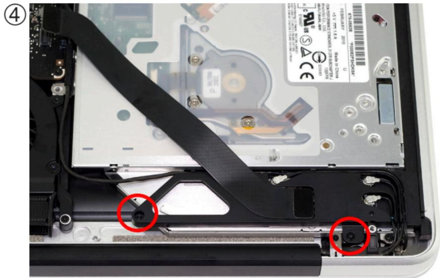
At the rear of the optical drive you will see an aluminum bracket that has a flexible ribbon cable and 3 Airport / Bluetooth antennas going into it. You need to release this bracket to access a screw underneath it, and also allow the optical drive to come out. Remove the 2 Phillips screws that are circled in red here. Note that one screw is substantially longer than the other.
