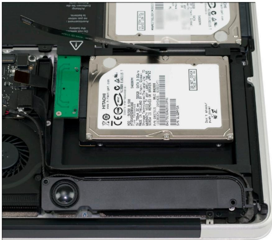
Here you see the OWC Data Doubler bracket inserted into the optical drive bay.
