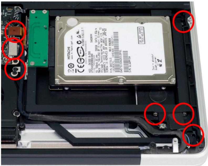
Installation of the OWC Data Doubler bracket with it's hard drive is the opposite of the disassembly process.
