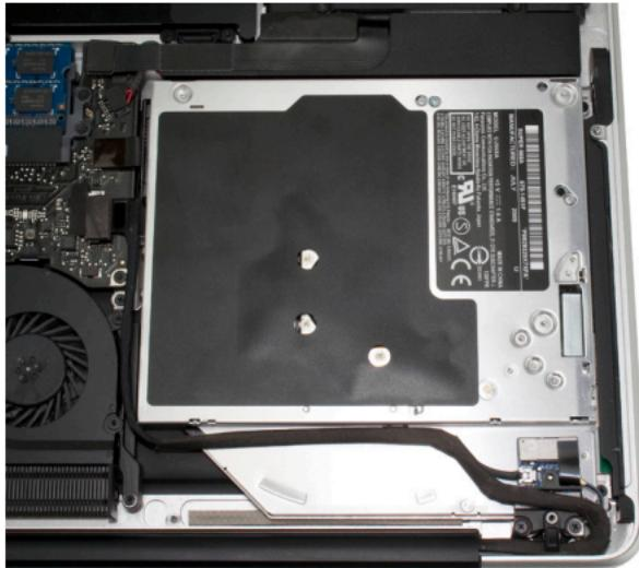
After you've taken the bottom cover off of the computer, you will see the optical drive that we will need to remove to install the OWC Data Doubler.
