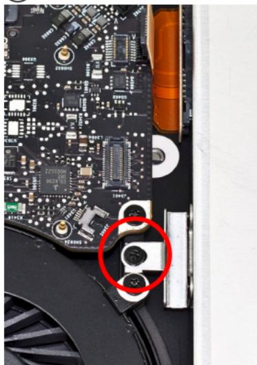
Once you have removed the small cable with the silver connector, underneath it you will see a silver metal bracket with a black Phillips screw in it that attaches to the back of the optical drive.
