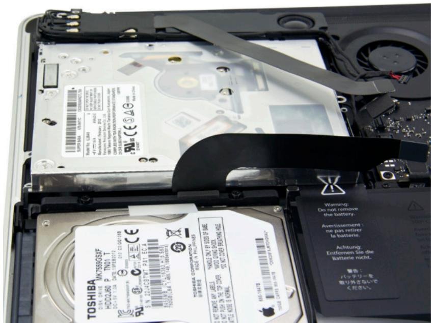
⑧ Gently lift the optical drive out of the bay, being very careful to not damage any cables in the process. The hard drive cable can be straightened up vertically as shown in this picture.
