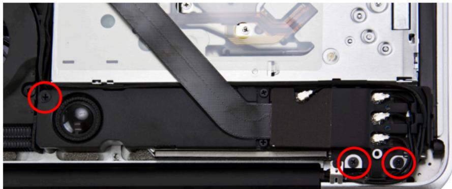
At the rear of the optical drive bay there is a black speaker assembly that has 3 Phillips screws that attach it to the chassis. Remove the 3 screws.
