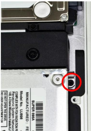
Once you have the final screws removed and the bracket with the antennas attached loosened, you can lift up on the optical drive from the area near the ribbon cable and gently wiggle it out of the chassis.
