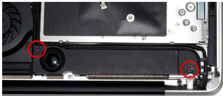
At the top of the optical drive you will see a speaker that has a wire running through a channel on it. Remove the 2 Phillips screws securing this to the chassis and gently lift the speaker away from the optical drive. You will not be removing it from the computer - it will stay attached. Don't worry if the cable comes out of the channel; you can just press it back in.
