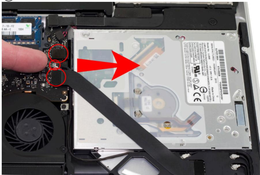
On the left side of the optical drive, you will see a two ribbon cables that are attached to the logic board with a small silver cable between them. You have to remove the small silver cable from the logic board. This is a delicate cable and it takes care to not damage it. Using your fingernail, gently pull the cable out of its socket, towards the optical drive to release it.
