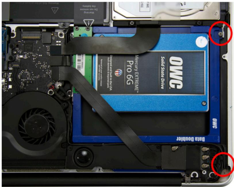
Install the OWC Data Doubler bracket by reversing the disassembly process.
