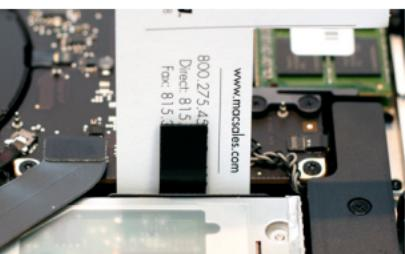
Here is another view of the business card fully inserted so that the edge is on the bottom of the chassis of the computer.
