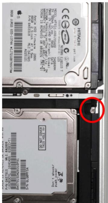
Install the OWC Data Doubler bracket by reversing the disassembly process.
