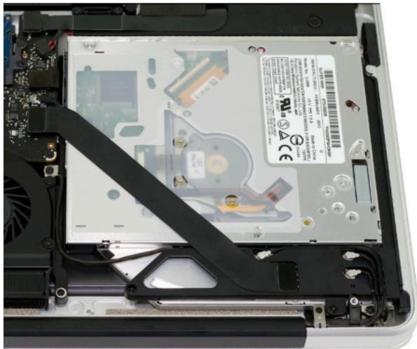
After you've taken the bottom cover off of the computer, you will see the optical drive that we will need to remove to install the OWC Data Doubler.
