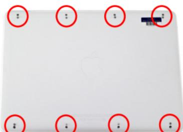
Place the bottom cover onto the laptop and replace the 8 Phillips screws you removed to take the bottom cover off.
