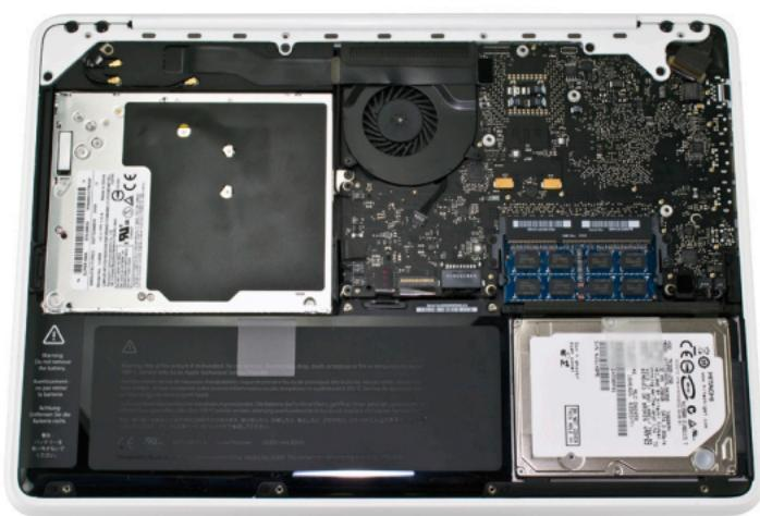
Remove the 8 Phillips screws securing the bottom cover on the laptop. All 8 screws are identical.
