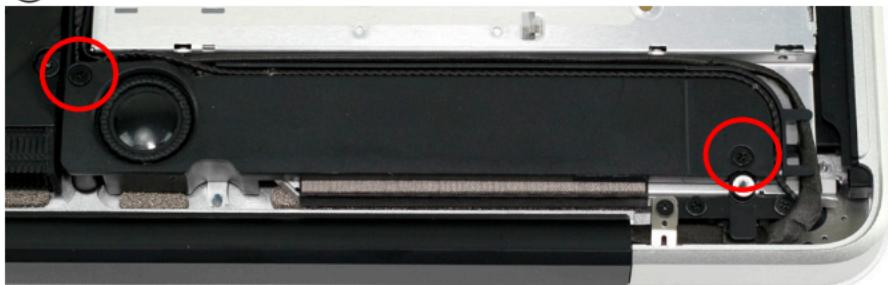
At the rear of the optical drive bay there is a black speaker assembly that has 2 Phillips screws that attach it to the chassis. Remove the 2 screws, noting that one is substantially longer than the other.
