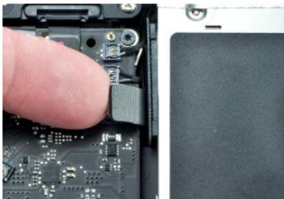
On the left side of the optical drive, you will see a black screw inserted through a silver bracket that is attached to the back of the optical drive. Remove the Phillips screw. Above the screw you just removed you will see an orange or black ribbon cable that connects to the optical drive. You need to lift up gently on the cable using a fingernail to release it from the connector on the logic board.
