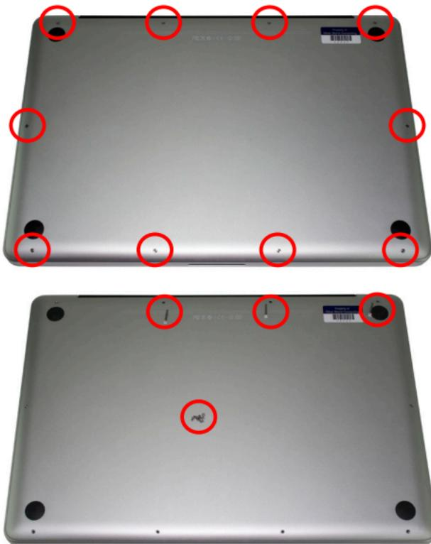
Remove the 10 screws that secure the bottom cover onto the laptop using a Phillips P0 screwdriver.
