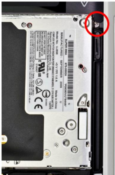
Begin removing the optical drive by taking out the silver screw at the top right of the optical drive. It's partially concealed by a black plastic tab that is part of the battery.
