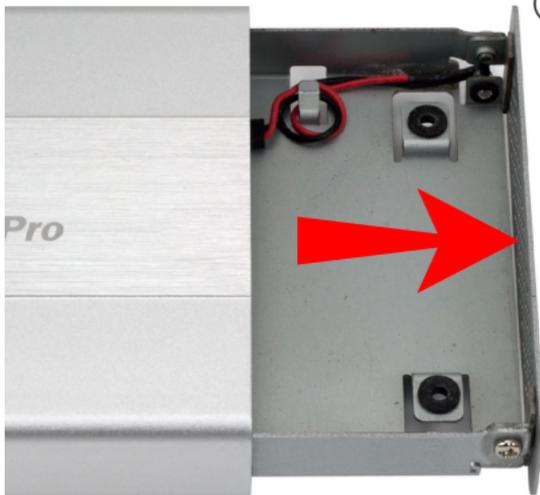
③ From the rear of the enclosure, press inwards on the rear ports to slide the inner chassis out towards the front of the enclosure.
