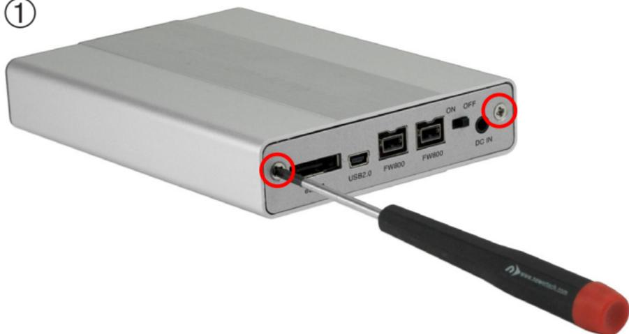
Use a Phillips P0 screwdriver to remove the 2 screws holding the rear backplane cover in place.
