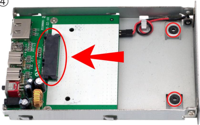
Once the inner chassis is removed from the outer enclosure, you will see the SATA data & power combo connector where your 2.5" SATA drive will attach to the bridge card.
