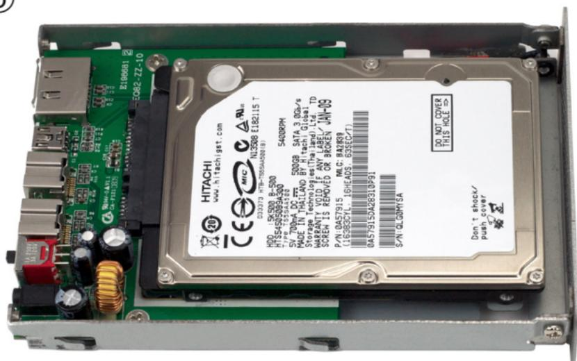
Place your drive mechanism into the chassis, lining up the connector, and slide the drive towards the ports to firmly affix the drive into the SATA connector.
