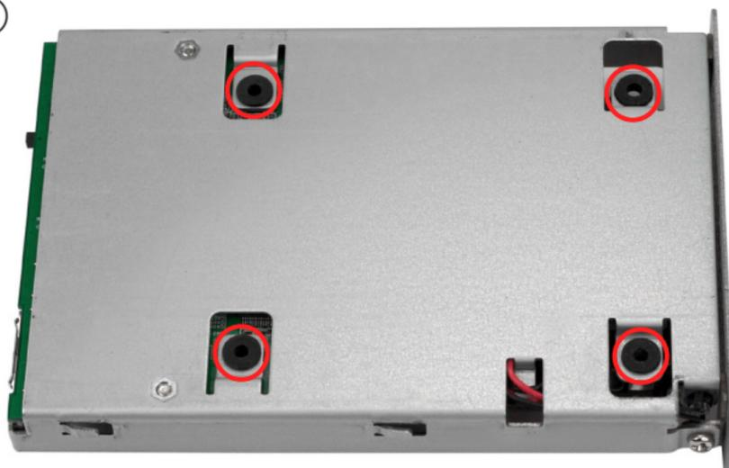
With your fingers holding the drive mechanism into the enclosure, turn it over so you can see the screw holes that you will need to use in the next step.
