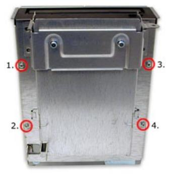
Insert the 4 screws shown here from the bottom of the CD drive carrier and you're ready to reinstall the new optical drive.
