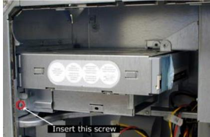
Insert the two Phillips screws you removed from the optical drive carrier.
