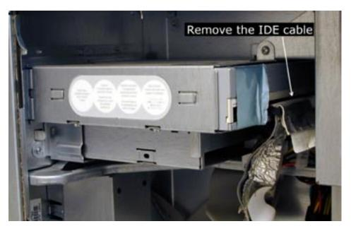
Begin by opening your system and touching a metal component such as the CD-ROM bay to ground yourself. Always be aware of static while working in your system, you can use a grounding wrist strap if you wish. Reach in and unplug the IDE cable from the back of the optical drive you are removing. If you have a ZIP drive installed, you will want to remove the IDE cable from it as well (not installed, and not pictured).
