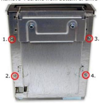
Remove 4 screws from bottom of drive
