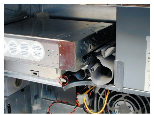
Slide the CD carrier back into the chassis fully, make sure the "ear" is through the hole as shown.
