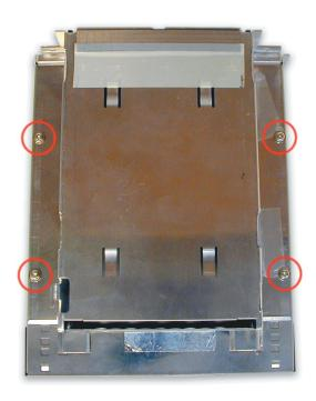
Remove the 4 screws shown here from the bottom of the CD drive carrier and you're ready to remove the old CD drive.
