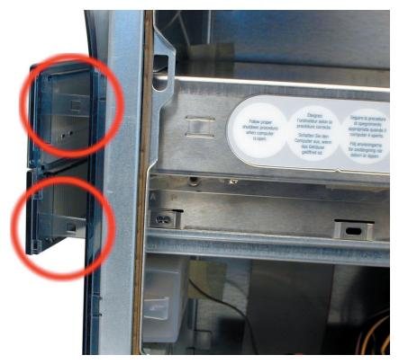
Look at the front of the computer and you will see 2 plastic tabs poking through the front of the case into the CD bay area. You will need to gently press these tabs toward the CD carrier to release them, and the double drive door will slide forward in it's mount as shown here. Remove the door from it's tabs on the opposite side.
