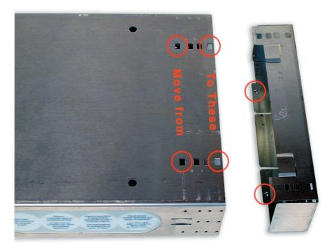
Remove the sheet metal end cap from the CD-ROM tray by lifting on the metal tabs circled on the endcap. You'll want to reinstall the endcap out to either the last set of holes, or the 2nd from last set. Once you install the new drive, you'll see where to place it.
