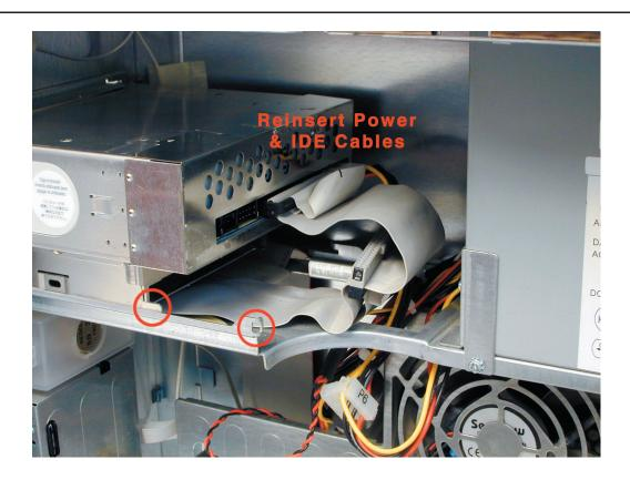
Slide the completed assembly back into the chassis as you removed it. Note the two red circles here, that is the "ear" that has to slide through the circled opening upon completion, it's there as a guide. Reinsert the power and IDE cables as you removed them (and hook up your ZIP drive if you have one, once again, not pictured).
