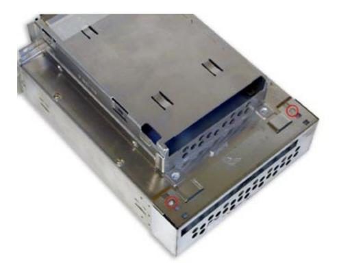
One more picture showing the 2 tabs attached in the proper position for the DVD-R mechanism install.
