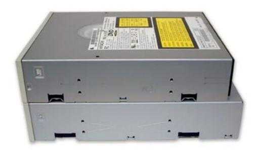
Set the old drive on top of the new drive (in this case, a DVD-R mechanism) and you'll see that in many cases, you will need to adjust the backpanel on the CD Drive carrier for depth.
