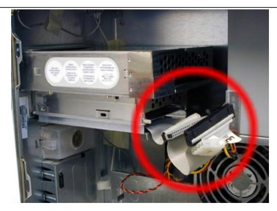
Reach in and gently remove the power and IDE cables from the back of your existing CD drive (and, if installed, your ZIP drive, not pictured). Lay them forward, out of the way, as shown.
