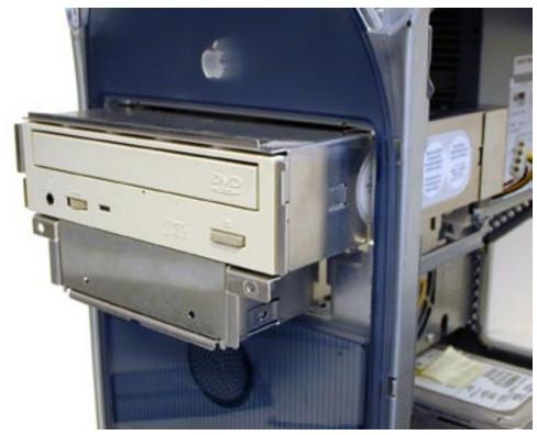
Once the two screws are removed, the CD drive bay will slide forward in it's track mount out of the computer. Remove it now, you may have to gently wiggle it up and down to free it from the bay because at the rear is a sheet metal endcap - it may get caught coming through the opening.
