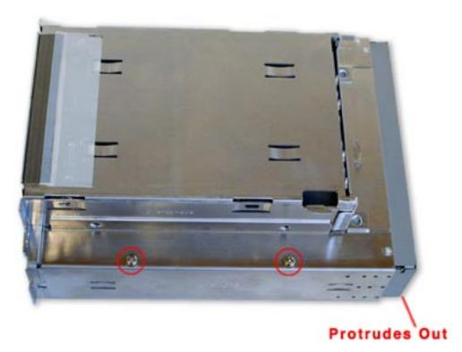
In this picture you can see how far the new DVD-R drive protrudes out from the drive carrier. The original drive fit flush, no protrusion at all. In this case, the 2nd from last set of holes will be used to replace the endcap. Also, once the drive is inserted, attach it to the carrier using the 4 screws you removed from the original drive (2 shown here).
