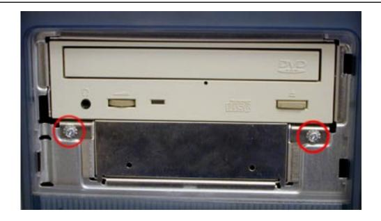
Look at the front of the computer where you removed the drive bay doors and you will see two phillips screws securing the bay into the computer chassis. Remove these two screws and set them aside.
