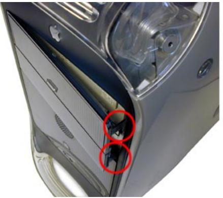
Reinsert the front double door panel back into the computer as you removed it. The two tabs that protrude into the CD carrier bay will need to be gently pressed inward to align with their slots. Once you do that, the double door simply snaps closed on the front of the computer.
