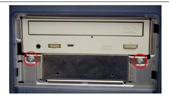
Replace the two screws from the front of the CD carrier.
