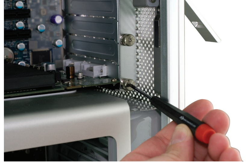
Using a Phillips P0 screwdriver, loosen the PCI Express cover retaining plate and remove it. There is a tab at the top that the metal plate latches into, you'll need to unscrew the 2 screws and slide the plate down out of the tab.
