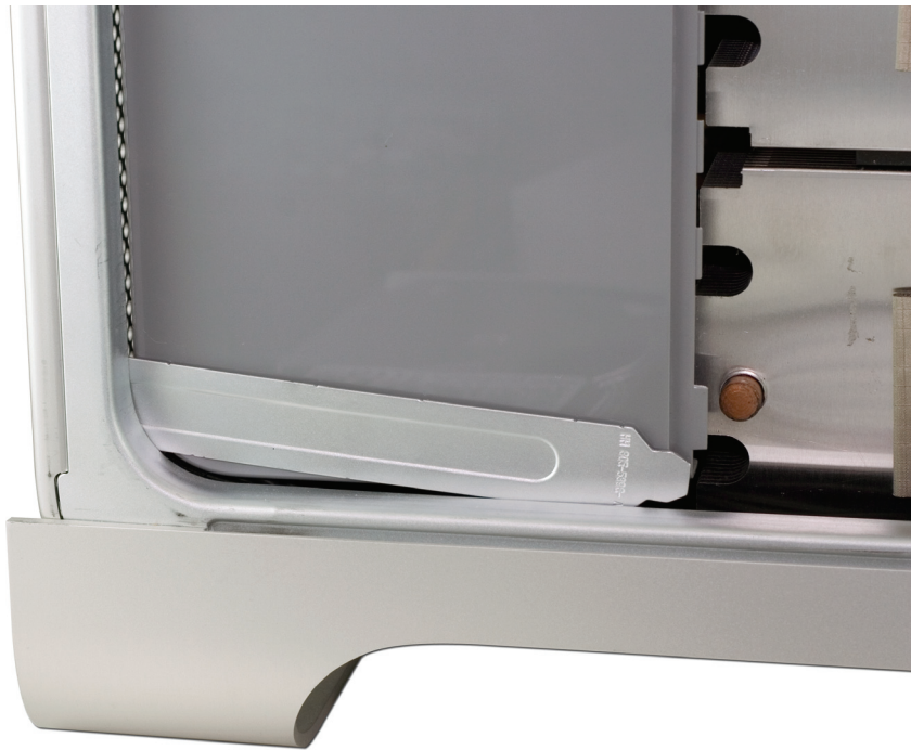
Take the L shaped PCI card deadplate and, starting at the top of the fan shroud, work the short end of the bracket into the gap at the back of the Mac Pro, as shown above.
