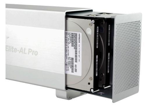
Slide the assembled chassis back into the enclosure from the front to the rear.
