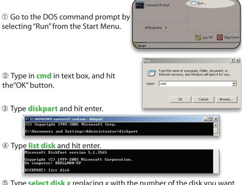
⑤ Type **select disk x** replacing x with the number of the disk you want to reformat. (Typically, you will see an asterisk (\*) under "GPT" for the disk requiring formatting.)
