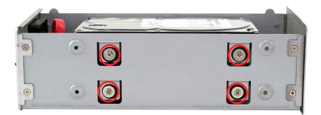
Secure the 2 hard drives into the chassis by inserting the 8 Phillips screws (4 each side) through the black rubber anti-vibration grommets, and into the hard drives. You may have to lift up a bit on the drives to get them into position. Firmly tighten the 8 screws to secure your hard drives into the chassis.
