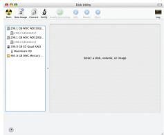
Select the device with no volumes attached to it; in this picture, that would be the 465.8GB OWC Mercury drive, your drive may be of a different size depending on the mechanisms you use. Click once on the picture of the drive icon next to the text.
