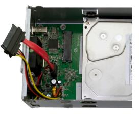
drive position, and connect one of the red SATA cables to the hard drive you are installing in the lower position, and place the hard drive into the chassis.
