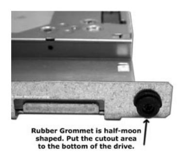
The two grommets / washers on the right side are universal in orientation, because they are round. The two grommets on the left side are half-moon shaped and the moon (larger portion) should be facing up as shown in this picture. The drive slides down onto the smaller portion of the grommet and if improperly installed, the case will not close on the PowerBook.
