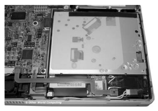
Upon removing the bottom shell of the PowerBook, you will see the optical drive on the left side of the computer. Turn the machine so the drive is oriented facing you, as shown in this picture. There are a number of cables and connectors you need to unhook to remove this drive. The cards attached to the drive brackets are a modem (left) and the inverter board for the display (right).
