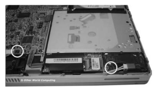
Detach the ribbon cable from the inverter board and then from the logic board - the two positions you remove the cable from are shown circled in this picture. Set the inverter ribbon cable aside.
