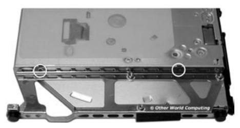
Remove the two Phillips screws from the large right metal frame. Notice that the screw on the left in this picture is a zero draft head - very flat, and it will need to be put back into this hole, otherwise the modem card will not fit flush back into place upon reassembly. Set the frame aside.
