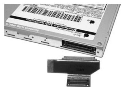
Remove the drive connector cable from the back of the drive and set it aside.
