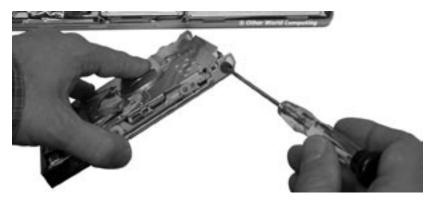
Use the Torx T-8 screwdriver to remove the 4 screws and grommets that are at the corners of the drive. You will notice that the screws are all identical, but there are 3 different types of grommets.
