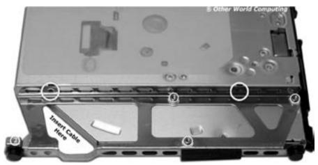
Begin assembling the new drive by placing the large right frame on the new drive. Attach the small zero draft screw on the left, and the regular screw on the right (circled with the large circles above). Gently slide the modem's ribbon cable through the slot shown above, placing the modem on the screw risers circled on the left. Do the same with the inverter board, placing it on the right, with the power connector toward the modem card.
