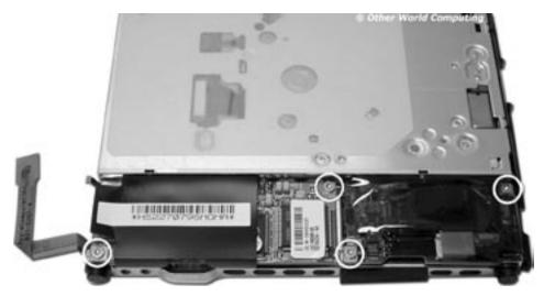
You are now ready to physically remove the drive from the PowerBook. Start by gently lifting up on the drive where the modem and inverter boards are at, angling the drive from the outside. The 2 rubber grommets that the drive rests on will allow the drive to lift freely on the outside, but not the inside. The inside grommets are captive and fit inside holes in the frame and you cannot lift from the middle of the computer.
