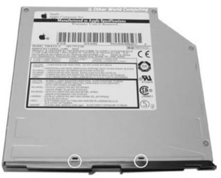
Turn the original drive on it's back and point the slot toward you as shown in this picture. Using a small thin straight screwdriver, or a paperclip, press gently on these two release tabs circled in this picture. You will find two more tabs on the bottom side of the drive (pictured below), and also one on the side. Once you release the tabs, you will see the other capture points and the removal is simple. Be patient, and do not break the tabs.
