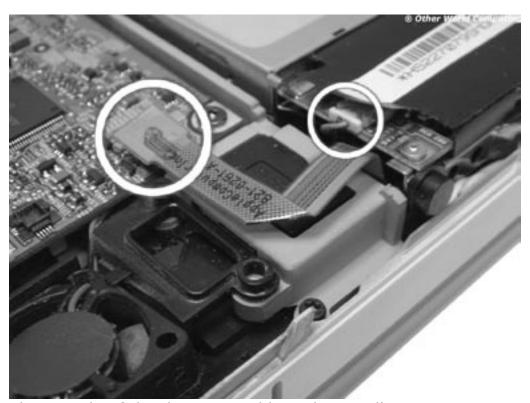
Look back at the outside of the drive assembly and you will see two more connectors that need to be detached. Unplug the ribbon cable from the logic board (it goes to the modem, underneath the drive), and also the 2 wire cable from under the edge of the black plastic cover on the modem card. That cable will need to be pulled straight out of it's connector toward the back of the PowerBook.
