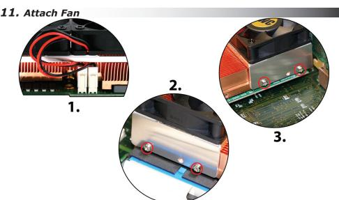
Plug the 2 fan connectors onto the CPU upgrade daughtercard. Insert the 4 included small Phillips screws through the holes in the fan assembly and attach to the heatsink in the location shown. You may need to remove the video card to insert the screws more easily. Some systems do not have enough clearance to screw in the screws hold the assembly without issue.
