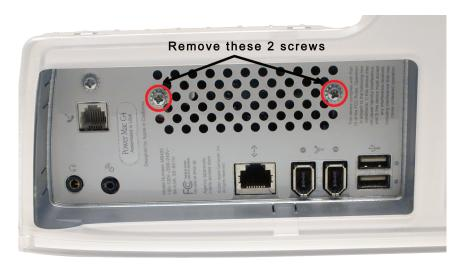
Unscrew these two screws from the rear port panel on your system. This will release the fan from behind the heatsink and allow you to unhook the rear heatsink clips in the next step. You will not be reinstalling this fan.
