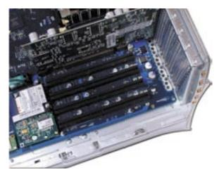
1. Locate an open PCI slot in your system.
