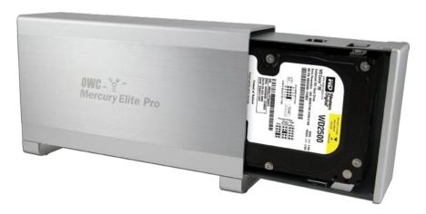
Slide the drive enclosure back into the outer shell, port end first into the case with the logo on the outer shell facing you, as shown in the picture.
