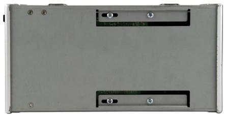
Turn the drive enclosure on it's side so you can access the bottom screws as shown. Install the 4 screws into the hard drive through the drive case.
