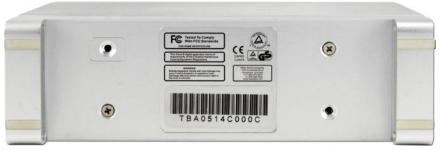
Turn the drive enclosure onto it's side as shown and remove the two Phillips screws that are inserted into the bottom of the drive enclosure. This will release the internal drive carrier. Slide the drive carrier out of the external housing, pushing it to the front.
