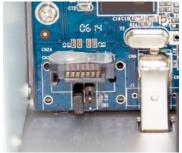
On the logic board of the dual bay case, you'll find a jumper that sets the configuration of the drive enclosure. By default, the case is set to span drives, allowing you to install 2 different sized hard drives. But with a simple jumper change, you
