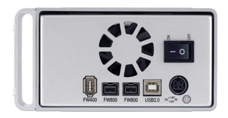
Turn the drive so you can see the rear ports. Connect the power cable to the back of the drive, and either the FireWire 400 or 800 cable to the drive, or the USB 2.0 cable (whichever you plan on using to connect to your computer). Plug the power brick into the AC power cable (not shown), and power the unit on. You should hear the drives spin up, and click a couple of times. After 10 or so seconds, the following dialog box should appear on your screen.
