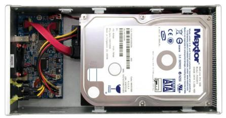
Turn the hard drive enclosure back over and insert the top hard drive. Insert the power and SATA cables into it, as you did with the bottom drive.
