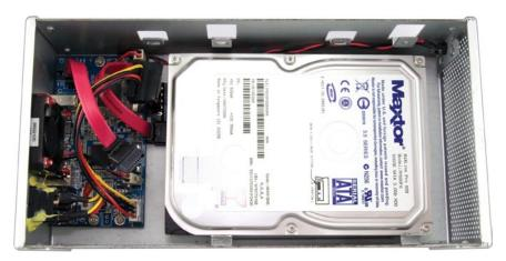
Place your first hard drive into the case, attaching one of the red SATA cables to the drive, and one of the red & yellow power cables as well. It's a tight fit so don't put excess pressure on any of the connections while performing this step.
