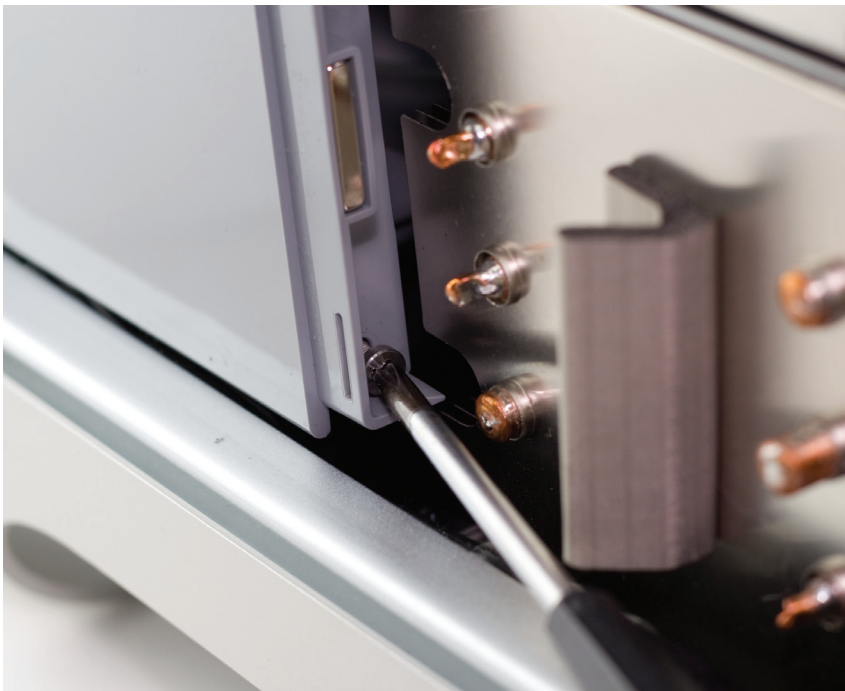
Some later model Mac Pro systems, especially 8-Core models, have a hidden Phillips screw located at the base of the fan assembly. Unscrew it.
