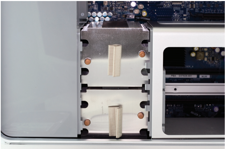
A view of the processor heatsinks with the cover removed.
