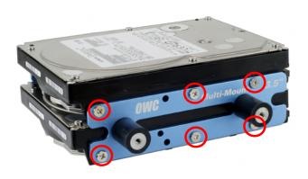
Begin by positioning the bottom 3.5" Hard Disk Drive (HDD) with the connection ports facing away from you, then pick up the drive bracket labeled as OWC Multi-Mount 3.5".
