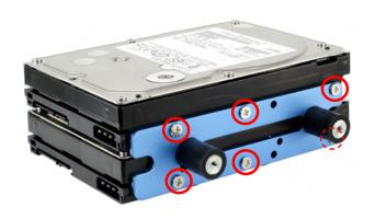
Once you have the right bracket installed, rotate the hard drive and attach the left side bracket using the same method described earlier.
