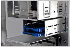
Here a typical PC case is shown with the 2.5" Multi-Mount brackets installed in both a 5.25" (top) drive bay, and also in a 3.5" drive bay (bottom).
