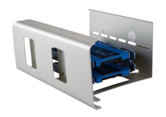
The Mac Pro's optical bay can support a total of two SATA devices. First, attach the completed Multi-Mount assembly to the optical drive cage using the four screws that Apple supplies (attached to the cage). Once the Multi-Mount is secured, start sliding the cage back into the optical bay, threading the large cutouts on the bottom of the cage with the large screws on the bottom of the bay.
