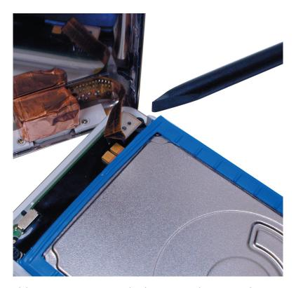
Another view of the ribbon connector, with the screwdriver tool pointing toward it. Do NOT remove the connector - it is not necessary to replace the battery.
