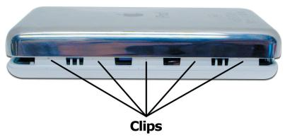
Using the included nylon screwdriver tool, gently insert the pointed end between the metal back casing and the acrylic front of the iPod, at the middle of the unit at the clip points shown. You will insert the tool from the face of the unit, pointed toward the back (metal) portion of the case. Once inserted, work the tool from the center of the unit, towards the top and bottom (left to right in this picture.
