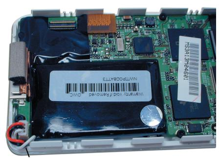
Insert new battery and make sure to route wires as shown - do not pinch them in the case!
