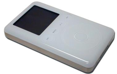
The back case snaps onto the front easily, just make very sure you don't pinch the wires from the new battery. Once that is complete, your iPod is ready to be charged! Make sure that you charge the battery for a minimum of 3 hours, uninterrupted. Overnight is better - once it's plugged into it's power adapter or FireWire port, you can go ahead and turn the unit on, if it didn't come on automatically by itself. You may need to perform a reset on the iPod, to do so follow these directions:
