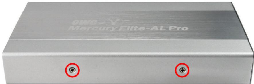
Once you have completed installation of your drive, turn the chassis so that the ports are on your left as shown in the above picture. You can see the 2 screw holes that the drive enclosure outer shell screws into circled. Slide the outer shell onto the inner chassis from the rear and insert the 2 Phillips screws you removed to start the assembly process. The enclosure is now fully assembled.
