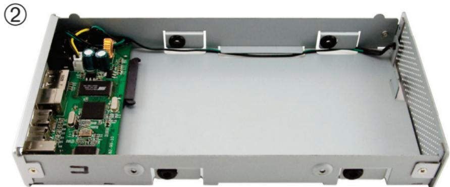
Here you see the OWC Mercury Elite Pro internal drive tray compartment. There will be a package of 4 screws inside of the compartment taped down, please remove them to use in step 4.
