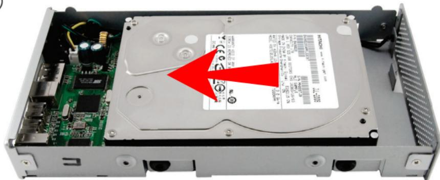
Place your drive mechanism into the chassis and onto the bridge card, and press the drive towards the ports to firmly affix the drive into the SATA connector. You may need to wiggle the drive from side to side to fit it in between the rubber grommets that the drive is secured with. Be sure to not tear them when inserting the drive into the chassis.
