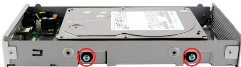
Insert (but not fully tighten) 2 of the included Phillips screws into the drive mechanism through the rubber grommets on the side of the enclosure. Repeat on the other side of the enclosure - there are 4 screws total. Once you have inserted all 4 screws into the drive you can fully tighten them.
