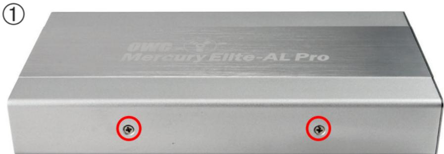
On the bottom of the OWC Mercury Elite Pro enclosure you will find 2 Phillips screws. Remove those two screws and the drive compartment will slide out towards the front of the enclosure. Remove the outer shell to proceed with drive installation.
