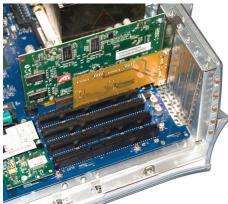
slot fully. Replace the Phillips screw.
