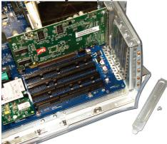
Step 2. Remove the backpanel cover from Step 3. Insert the OWC Serial ATA PCI card the PCI slot you want to use. Unscrew the into the slot - snapping it down into the Phillips screw and set it aside.
