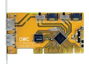
Open the anti-static bag and remove the OWC Serial ATA 2 channel PCI controller card. Take a few moments and examine some of the unique features of this card. You will need to configure the Serial ATA PCI card to work with your system before installing it.
