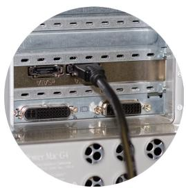
Internal Serial ATA (SATA) drives are also very simple to hook up. SATA drives connect using a keyed cable so you can't attach it backwards. Plug the SATA cable into the active port and then to your hard drive. Hooking up external Serial ATA (eSATA) drives is very simple. Just plug in the cable that came with your drive into the port that you have set up as being active. eSATA is keyed to only fit in one direction.
