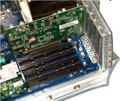
**Step 1.** Open your computer, and find an empty PCI slot. Clean out any dirt or dust that you see before proceeding.
