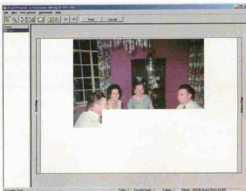
Figure 2. Running out of RAM can create more problems than just slow performance, especially on 32-bit systems. A common symptom of RAM shortages is partial rendering of photographs you're trying to print.
