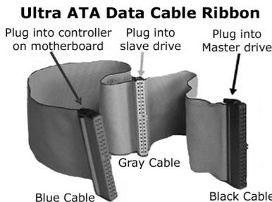
Please note the configuration of the internal ATA cable already installed in your existing system. If your internal cable is configured differently than pictured here, you may want to replace it before installing a new hard drive to achieve maximum performance.
