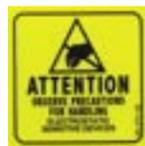
**ATTENTION!** While performing these upgrade procedures, static safe conditions must be met. Do not walk around, hold all components by their edges, and do not touch the connector contacts.
