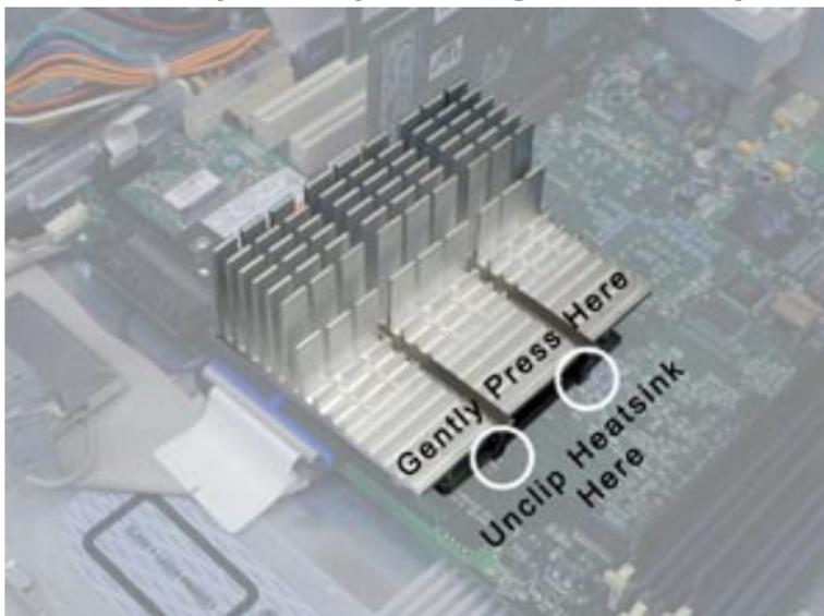
Remove the heatsink from your logic board. Use the needle nose pliers to unhook the clips from the processor card. **Skip to step 7 to remove the processor card.**
