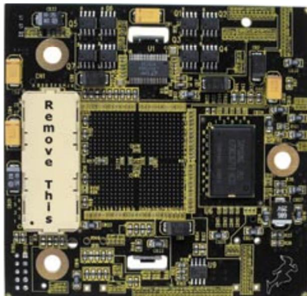
Remove the protective cap from the OWC Mercury Extreme G4 processor upgrade. The cap is located on the bottom of the card, between the screw holes. Place the cap onto the processor card you just removed.
