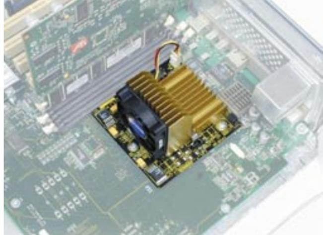
Installation of the processor daughtercard is the same on all systems, align the 3 screw holes in the card and gently place over the logic board. Firmly press straight down on the two rearmost screwholes until you feel the card "click" into place. Insert 3 Phillips screws into the 3 screw holes. **NOTE:** Do NOT press on the heatsink! You're all done - Enjoy!
