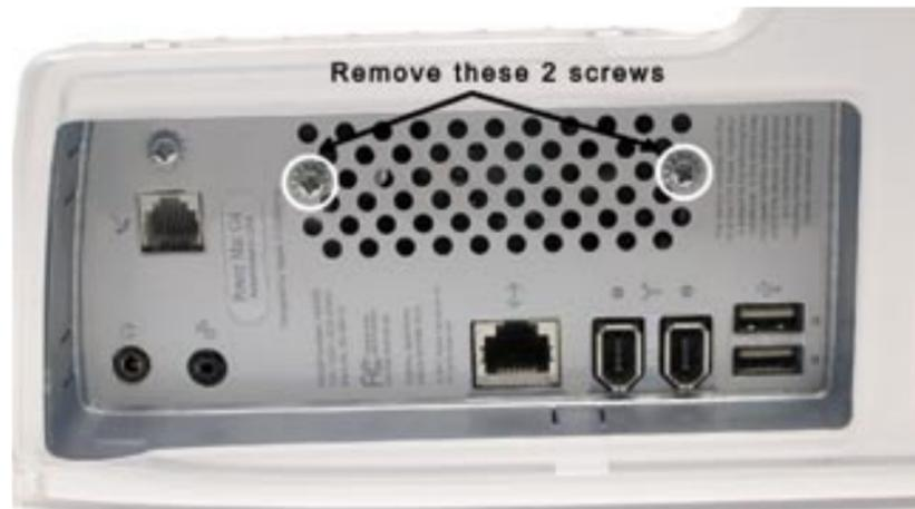
Unscrew these two screws from the rear port panel on your system. This will release the fan from behind the heatsink and allow you to unhook the rear heatsink clips in the next step.
