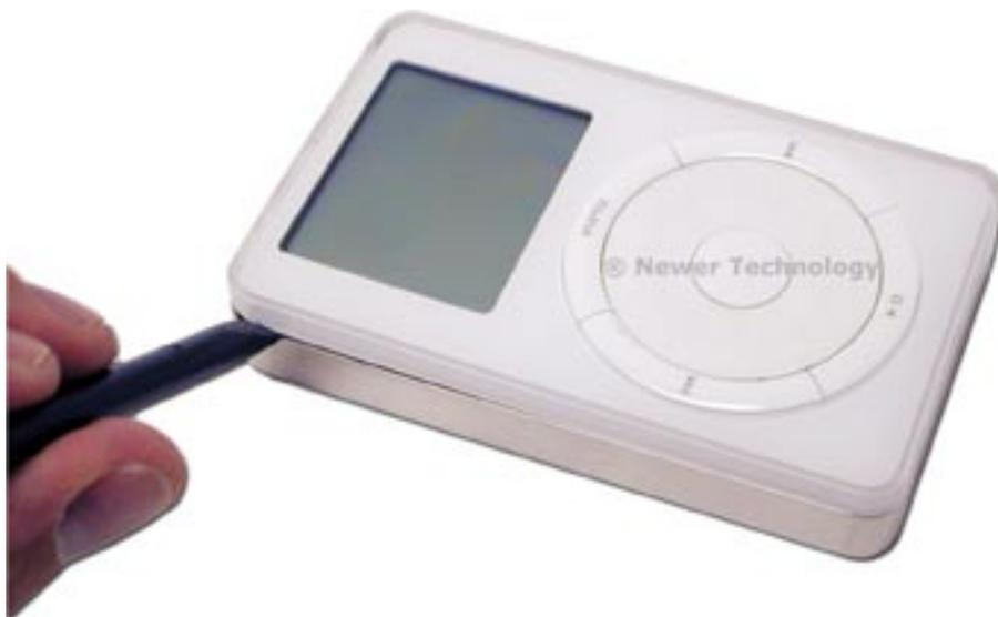
Using the included nylon screwdriver tool, gently insert the pointed end between the metal back casing and the acrylic front of the iPod, at the top of the unit as shown.
