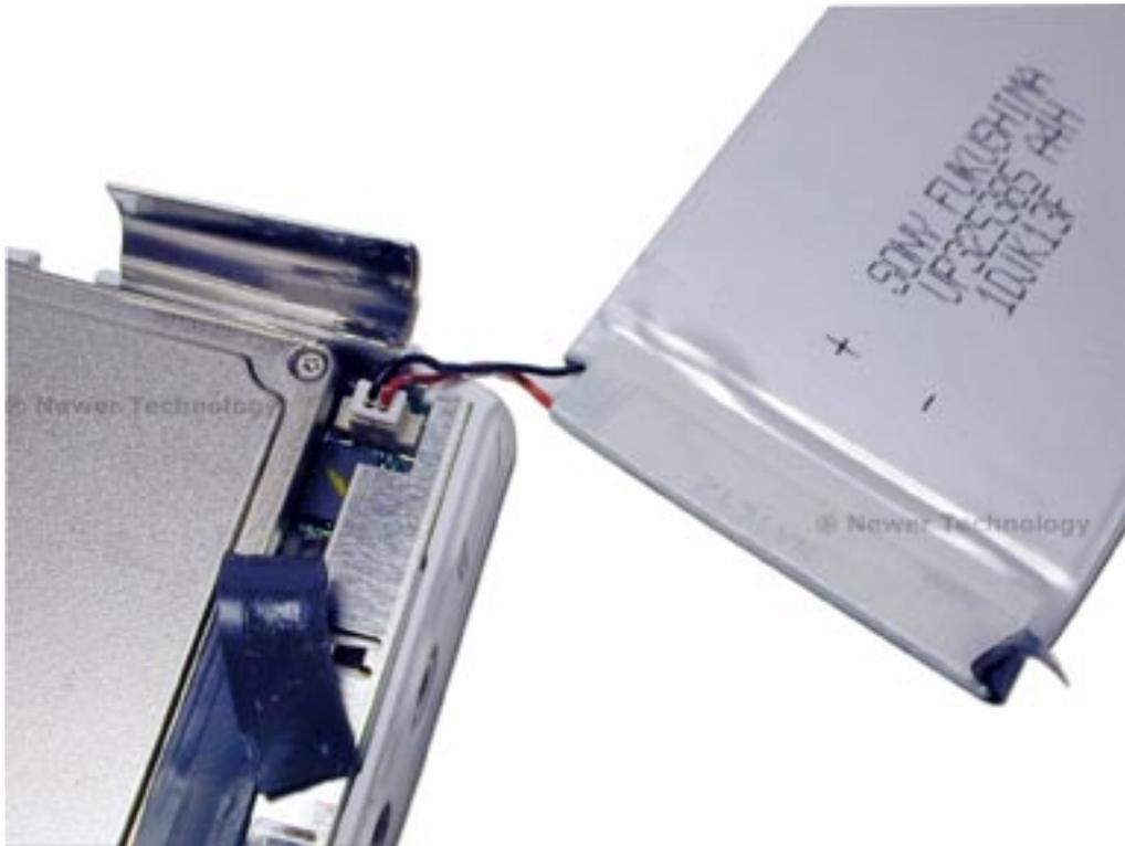
Disconnect the battery from under the top adhesive strip, from its mounting point on the logic board.
