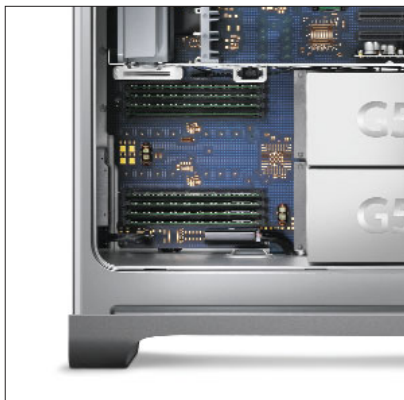
With the removable side panel, DIMM slots are easy to access.
