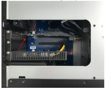
4. Remove the screw from the OEM controller card's bracket.
