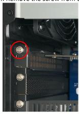
5. Before removing the card you need to position it so you can disconnect the two cables at the back. First, carefully lift the card out of its PCle slot and angle it as shown.
