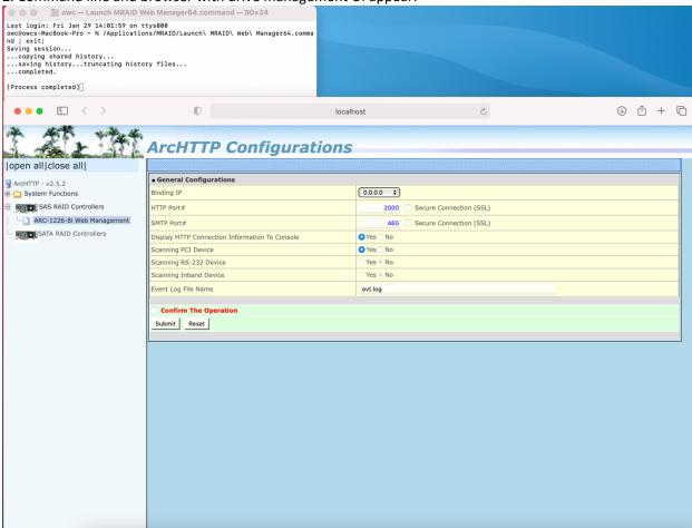
3. Click into the installed device environment, selecting the applicable option and drives to create an array. Note that the number of drives supported by each card can vary. This Areca card supports the full complement of 8 drives installed in the ThunderBay Flex 8.
