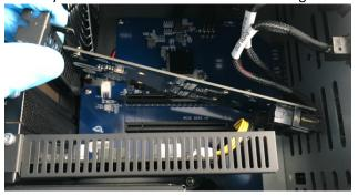
6. Next lift the front side of the card upward so that you can then lift the entire card out of the compartment.
