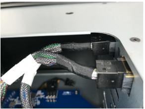
9. Pick up the RAID/SAS card then, making sure the cable with the gold paint mark on it is attached to the top connector, connect both cables to the card.
