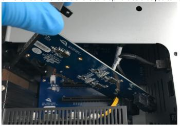
7. Letting the card rest at an angle so there is minimal tension on the cable connections, locate the tab on each connector (highlighted), then press down and pull the cable connectors back. Minimal force is required.
