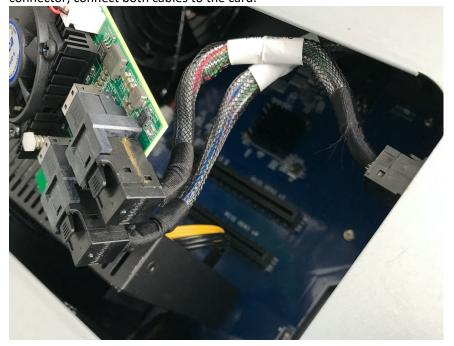
10. Carefully angle the back of the RAID/SAS card down into the PCIe compartent (at a similar angle and position as when you removed the OEM card in Step 6), then lower the rest of the card into the comparment. Last, re-align the card so that it can be seated in the PCIe slot as shown below.
