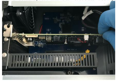
11. Carefully press the card into the PCle slot, making sure the rectangular notch on the front of the bracket (highlighted) aligns with the small tab on the case. This will ensure the bracket remains positioned so that the cutout for the screw aligns with the hole on the case. Due to the tension from the cabling, it is normal for the card to sit at an angle once seated in the PCle slot.
