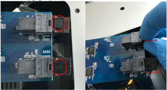
8. Set the card aside but leave the cables connected to the side of the PCIe compartment.
