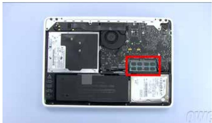
4. a. To begin removing the original memory, simply push outward on the two retaining arms until the top module pops up.
