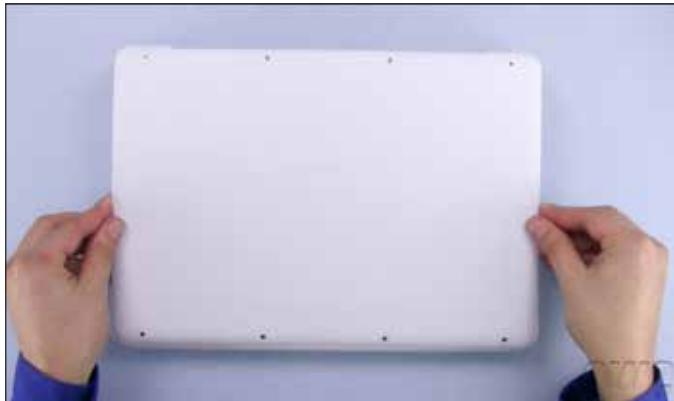
9. Using a Phillips screwdriver, replace the 8 screws that hold the bottom cover in place.
