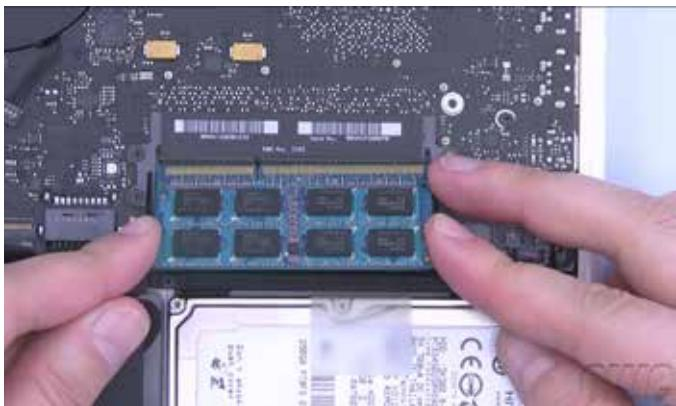
5. Repeat the process for the lower module. You may need to push on the retainer arms twice to eject the memory completely.
