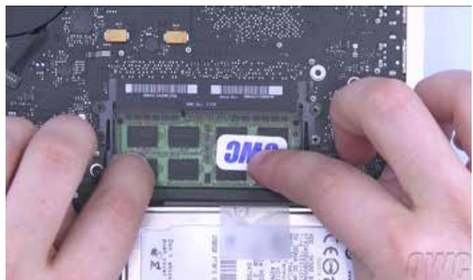
7. With the lower memory module installed, repeat the process with the top module.
