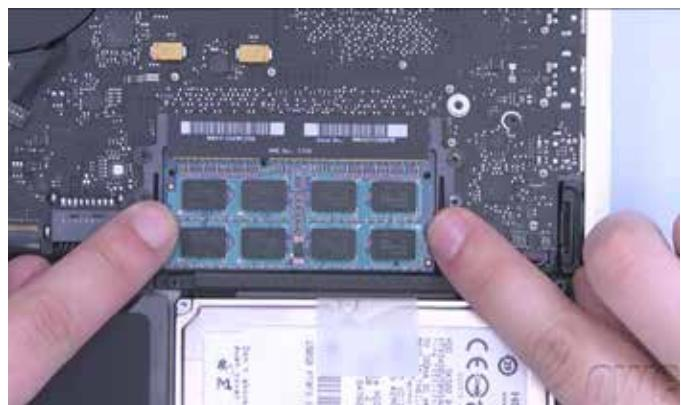
b. You can then slide the module straight out of the slot.
