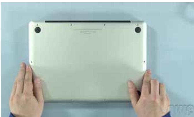
**13.** Using a Phillips screwdriver, secure the bottom cover starting with the 3 longer screws in the upper right.
