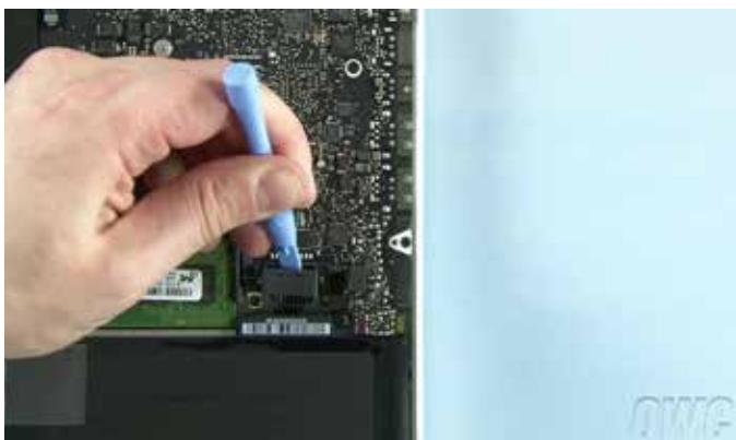
7. **a.** With the battery disconnected the memory can be safely removed. Simply push out on the two retaining arms until the top module pops up.
