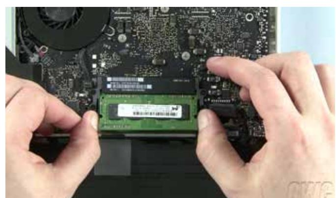
**b.** You can then slide the module straight out of the slot.
