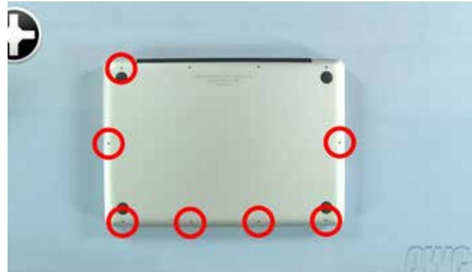
5. **a.** The bottom cover can now be removed. Starting near the hinge edge, simply lift up on the bottom cover and set it aside.
