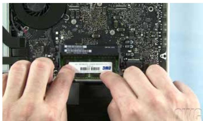
10. With the lower memory module installed, repeat the process with the top module.
