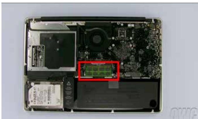
7. a. To begin removing the original memory, simply push outward on the two retaining arms until the top module pops up.
