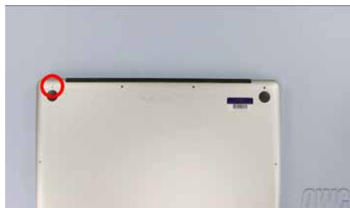
5. Finally, remove the remaining 6 screws which are also shorter.
