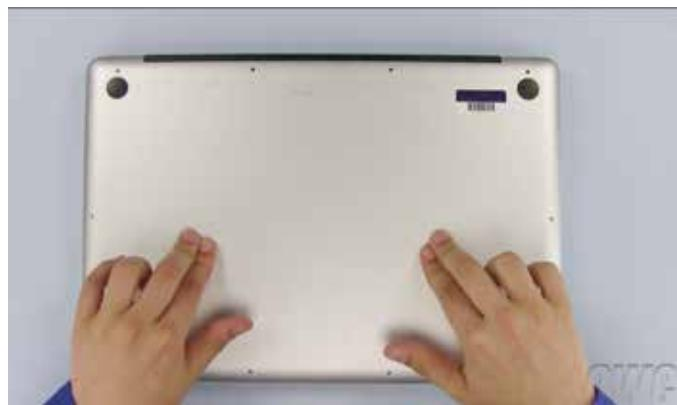
12. Using a Phillips screwdriver, secure the bottom cover starting with the 3 longer screws in the upper right.
