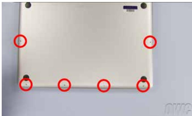
6. a. The bottom cover can now be removed. Starting near the hinge edge, simply lift up on the bottom cover and set it aside.
