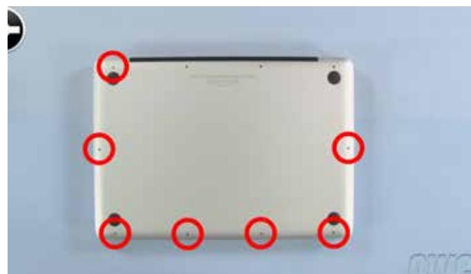
5. The bottom cover can now be removed. Starting near the hinge edge, simply lift up on the bottom cover and set it aside.
