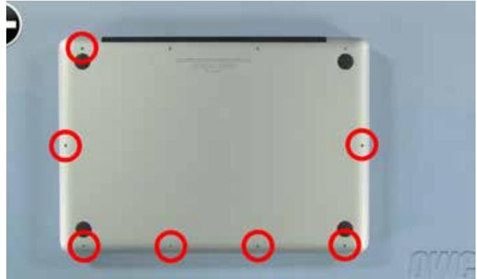
19. Once the bottom cover is secure, the MacBook Pro can be flipped over and powered on. The installation is now complete!
