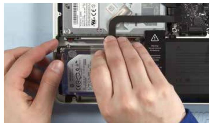
You can then unplug the SATA connector from the drive and remove the drive from the system.
