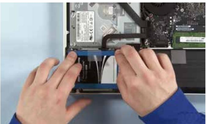
14. Next, replace the retainer bar and tighten the 2 Phillips screws that hold it in place.
