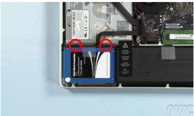
15. Finally, reconnect the battery by gently pushing its connector back into its socket.
