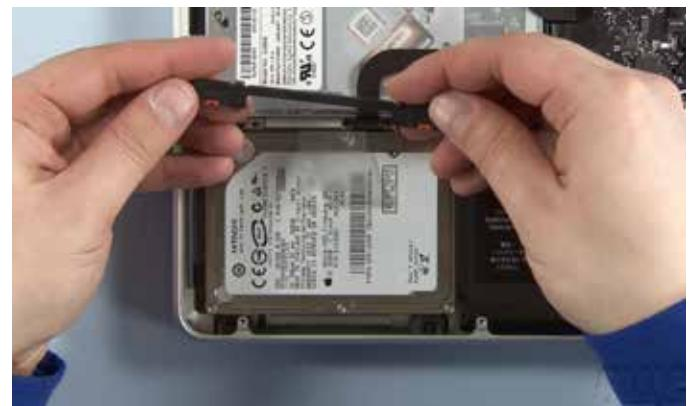
8. Next, pull the drive out of the bay by lifting up on the pull tab.
