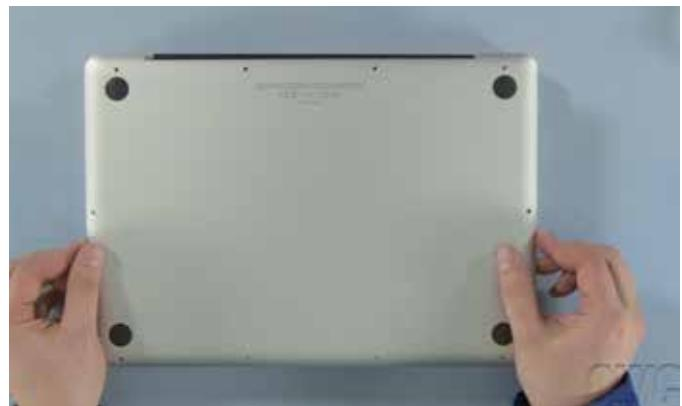
17. Using a Phillips screwdriver, secure the bottom cover starting with the 3 longest screws in the upper right.
