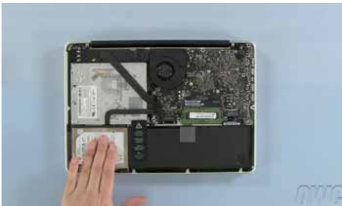
6. First, carefully detach the battery connector using a nylon pry tool.
