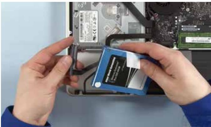
Then slide the drive into place making sure that it lays flat within the drive bay.
