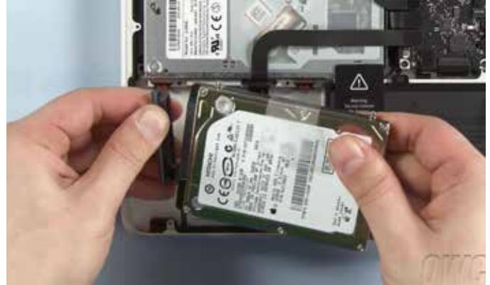
9. Using a Torx T6 screwdriver, remove and set aside the 4 mounting pins from the original drive. There are 2 pins on either side.
