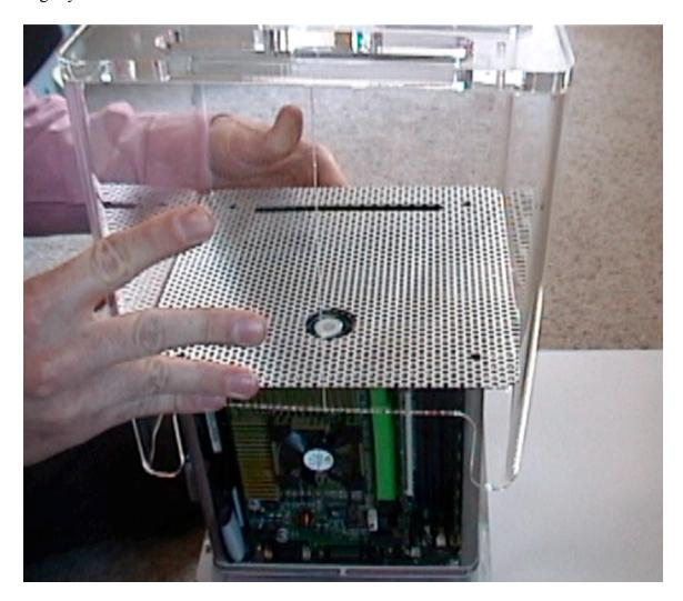
Make any minor physical adjustments so that the grille and ClearCube align properly, and tighten the screws using the Torx screwdriver.
