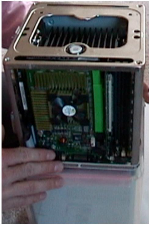
Take the grille and place it on the top of the Cube core. Align the four holes in each corner of the grille with the screw holes on top of the Cube core.
