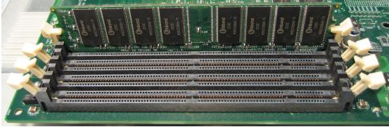
Look at the memory slots in your computer and make sure that they are clean - use compressed air to blow any dust out of the slots before proceeding. Open the clips at the end of the memory slots as shown to prepare for memory installation.
