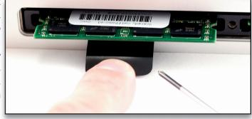
Slide the new RAM into your iMac's memory slots, one piece at a time until you feel resistance. The RAM should be nearly all the way in. Then, using your thumbs, snap the RAM into the computer fully - you will feel a "crunch" when it is fully installed.
