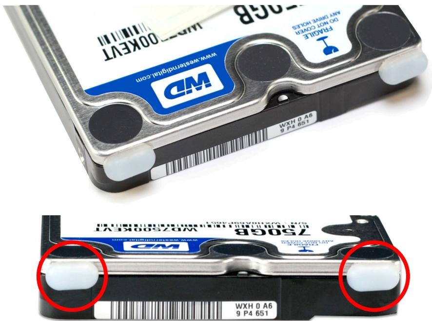
On the end opposite the SATA connector on your 12.5mm hard drive, place two of the silicone rubber feet on the top left and top right of the drive, at the highest point possible. These feet will keep the drive from moving around, and also aid in shock protection in case the drive is dropped.
