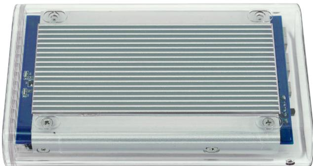
Insert 4 more 3.5mm screws into the bottom of the On-The-Go enclosure - you may need to put pressure on the bridge card to get all 4 screws to fully start. Then, turn to page 9 of the assembly guide to complete the installation.
