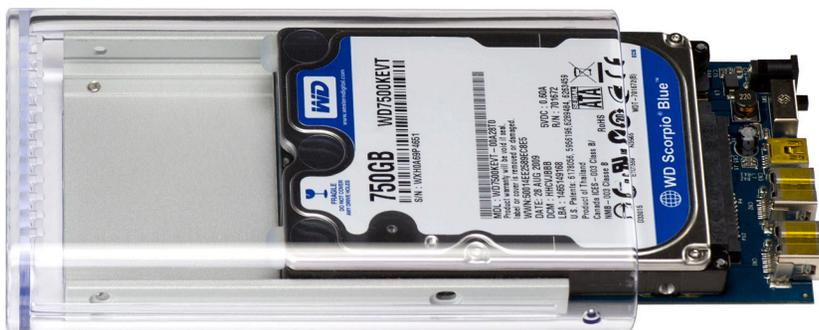
Slide the assembled bridge board with hard drive into the heatsink. Be very careful not to peel the silicone rubber feet off that you installed in step 6.
