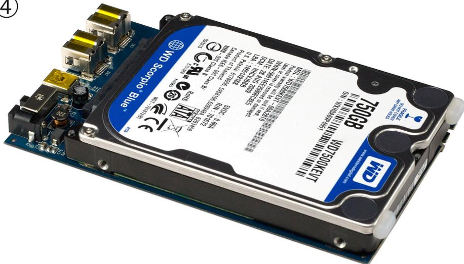
Insert the 12.5mm SATA Hard Drive on to the bridge card and onto the SATA connector on the bridge board, firmly seating the drive onto the connector. This is also explained on Page 7 of the full assembly guide.
