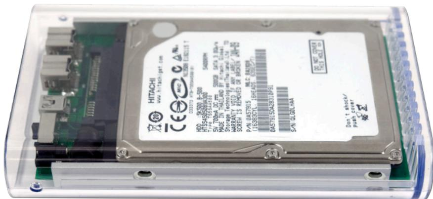
Here you see the OWC Mercury On-The-Go Pro drive inserted into the acrylic enclosure, ready to have it's end cap attached.
