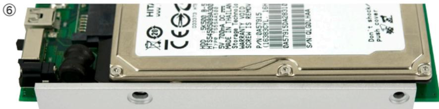
Slide the bridge card with the hard drive into the aluminum heatsink - there is a notch that the bridge card will slide into.
