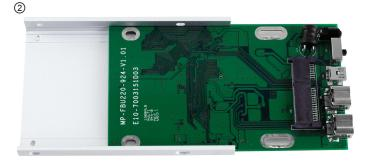
Remove the bridge card from the aluminum heatsink. It just slides in, no screws are holding it in place.
