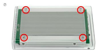
Gently slide the completed heatsink, drive, and bridge assembly into the acrylic enclosure.
