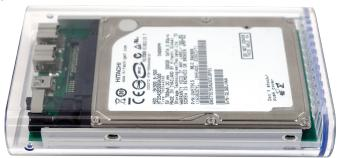
Here you see the OWC Mercury On-The-Go Pro drive inserted into the acrylic enclosure, ready to have it's end cap attached.
