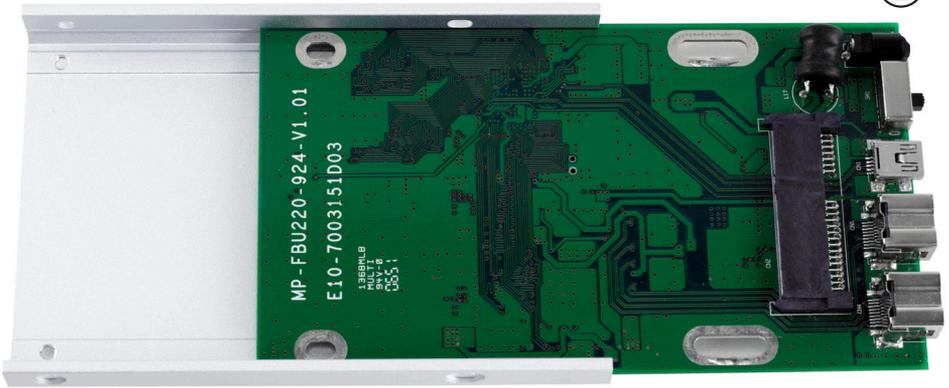
Begin by removing the bridge card from the aluminum heatsink. It just slides in, no screws are holding it in place.
