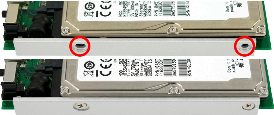
Slide the bridge card with the hard drive into the aluminum heatsink - there is a notch that the bridge card will slide into.
