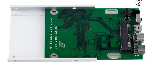
Begin by removing the bridge card from the aluminum heatsink. It just slides in, no screws are holding it in place.
