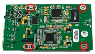
Turn the bridge over and look through the screw holes. Make sure they are fully lined up and insert 4 screws into the hard drive.
