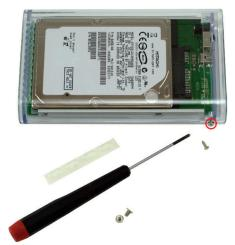
Insert the acrylic endcap, fully sliding it over the bridge card ports.
