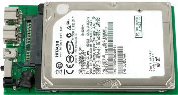
Place your hard drive mechanism onto the bridge card and fully seat the drive onto the connector.
