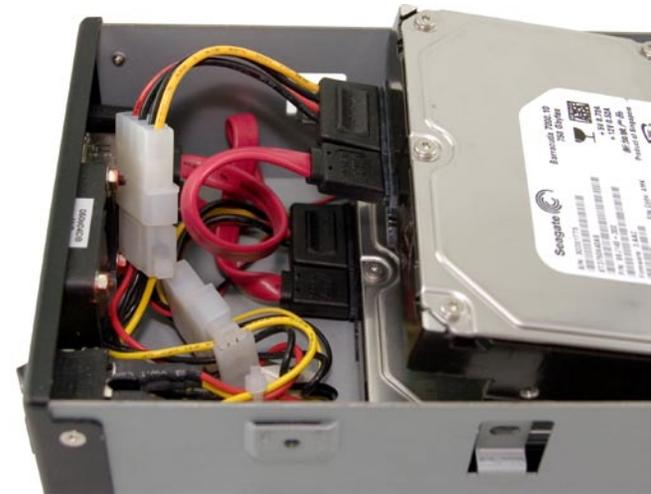
Repeat the procedure for the top hard drive, again, making sure you have not pinched any wires. Attach the power and data cables, and lower the drive completely into the chassis top drive bay.
