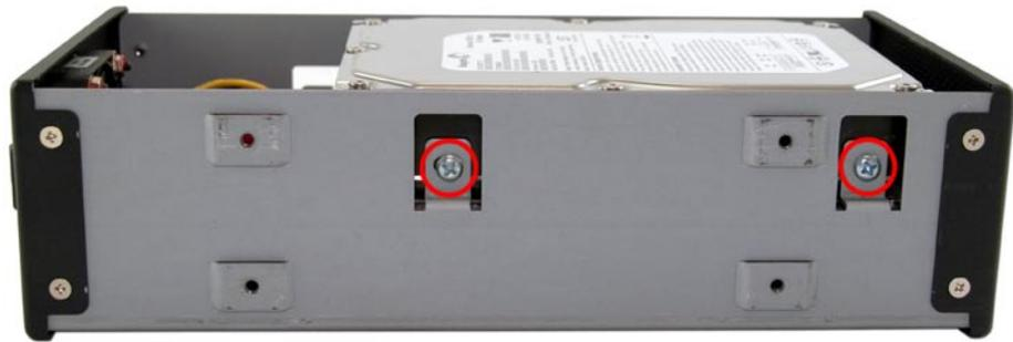
Attach your other 4 drive mounting screws to the top drive through the chassis on the top and bottom screw holes, as shown. Firmly tighten these screws as well.
