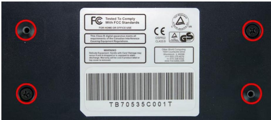
Once you have the drives fully installed, slide the chassis back onto the enclosure frame, and line up the bottom holes. Using the included screws, attach the chassis to the frame firmly.
