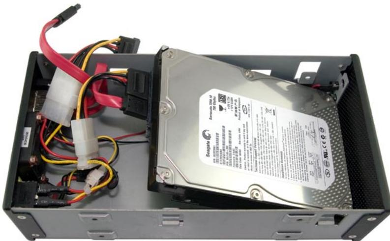
Insert the first drive mechanism into the chassis as shown. Make very sure that you do not pinch or cut the LED wire underneath the drive mechanism; you may need to use a screwdriver to route it around the drive mounting bracket. Attach the Serial ATA power and Serial ATA Data cable to the back of the hard drive as shown.
