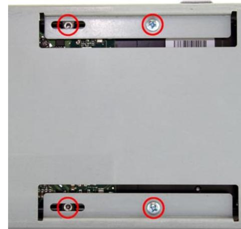
Lower the hard drive down into the chassis fully - and once again making certain you have not pinched any wires, line up the side screw holes and attach your mounting screws through the chassis and into the drive as shown. There are 4 to install, make sure they are all snug.
