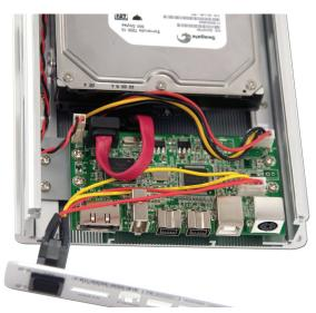
6. Once you have the cables attached, lower the hard drive down into the enclosure, until it is flat on the mounting rails. Make sure that the cables you just attached to the drive lay down flat, to aid in the last step when you slide on the top cover.
