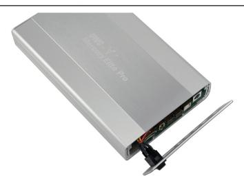
9. Set the top cover back onto the drive enclosure, sliding the cover onto the enclosure in it's enclosed rail. Once the top cover is fully closed, replace the 4 Torx T-10 screws from the back cover, and the drive is ready to hook up to your computer for formatting. Attach the power cable, the interface cable of your choice, and power the drive on.
