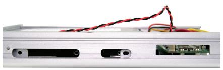
7. Look at the side of the drive enclosure. You will see the 2 holes shown here, on each side of the enclosure. Fasten the drive into the enclosure with the included Phillips screws here.
