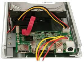
5. Take your 3.5" SATA hard drive and set it into the drive enclosure. You need to attach the power cable (the red, black, and yellow cable) to the SATA hard drive, and also connect the SATA cable to the hard drive. Make certain that you do not pinch the red and black LED cable on the left side in this picture - make sure it's free from being caught underneath the drive.
