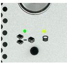
The front of the OWC Mercury Elite-AL Pro Dual-Drive solution has 2 LEDs on it that you should recognize. The right yellow LED shows drive activity - and will flash or remain steady while you are reading or writing to the OWC Mercury Elite-AL Pro Dual-Drive solution.
