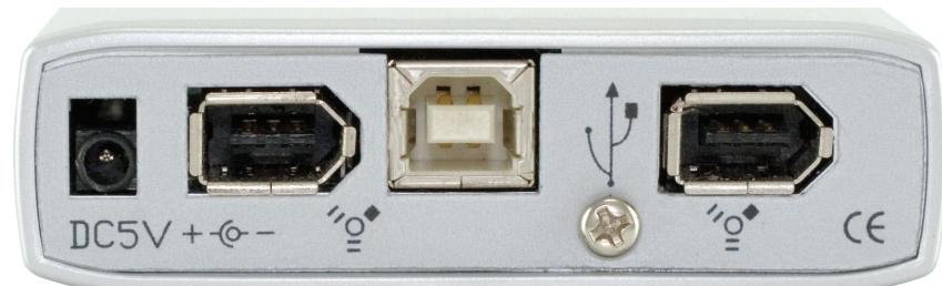
There is no power switch on the OWC Mercury Express drive, to power off the drive, you need to physically pull the cord out of the DC power port, or unplug the Firewire or USB cable from the back of the drive.
