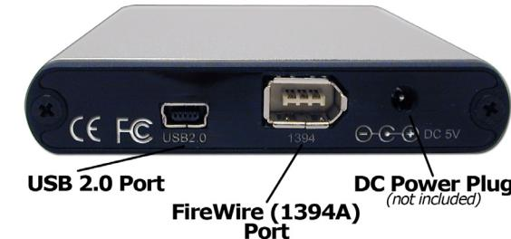
There is no power switch on the OWC Mercury Express FireWire drive, to power off the drive, you need to physically pull the cord out of the DC power port, or unplug the FireWire cable from the back of the drive.
