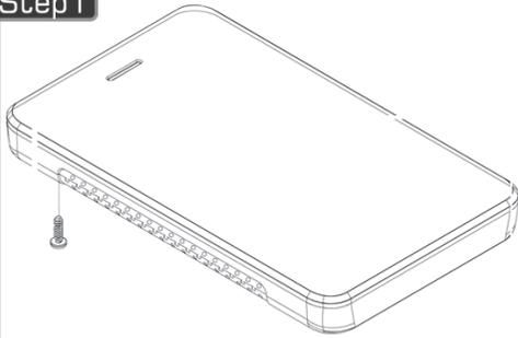
Remove the 2 Phillips screws from the bottom of the enclosure.
