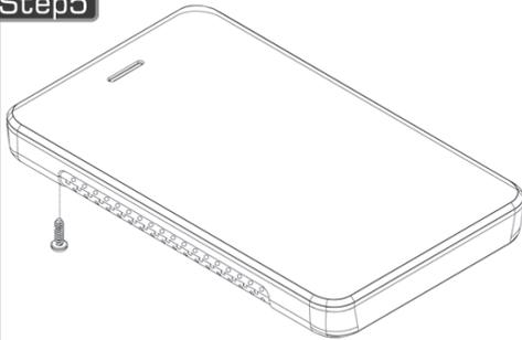
Replace the 2 Phillips screws from the bottom of the enclosure.
