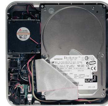
**3.** Place the drive and bracket inside the Newer Technology miniStack v2 enclosure, routing the power and ATA cables to avoid pinching them. The ATA cable will need to be folded at a 45 degree angle once it's set into the drive enclosure.
