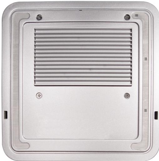
**1.** Begin by removing the 4 Phillips screws from the bottom of the Newer Technology miniStack v2 enclosure. Remove the drive carrier from inside of the Newer Technology miniStack v2 enclosure.
