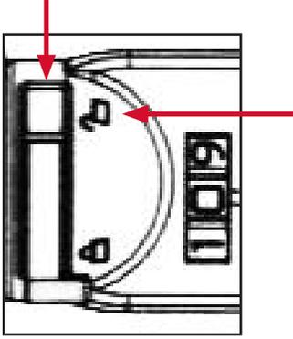
**Step 8** - To set the lock, insert it into the device's Kensington Security Slot, then set the lever to the closed position. Next, change the combination to a random number. The lock should now be secured to the device. Test the lock lever. If it will not slide to the open position, it is securely locked.
