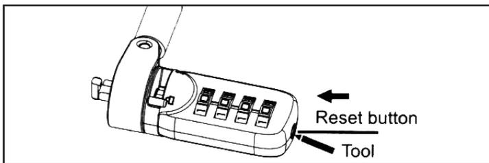
**Step 3** - While holding in the reset button, set a new four digit combination, making sure to align the numbers with the combination notching line as you did in Step 1.
