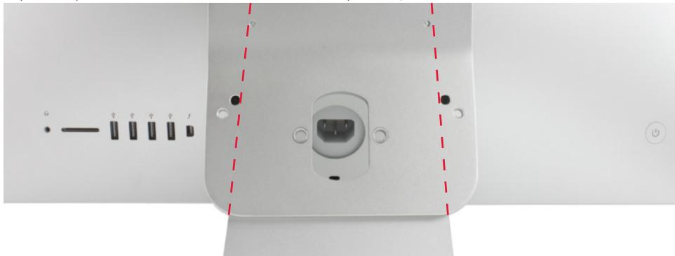
3. Use the clamp to secure the NuMount VESA adapter to the iMac stand. Place the clamp in the hole in the iMac stand with the rubber O-ring on the clamp facing the adapter. Line up the screw holes in the clamp with the screw holes in the adapter and use the included hex key and the longer socket-head screws to fasten the clamp to the adapter. The following set of pictures shows this process from the front, side, and rear respectively.
