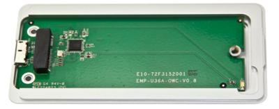
3. Insert the SSD into the black connector (circled below-left). The connector is notched so that the SSD fits using only one orientation. Next, use the short Torx T5 screw to hold the SSD in place (circled below-right). Do not over-tighten the screw.
